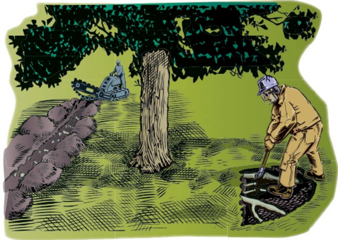
Figure 1. Selective root pruning consists of soil excavation prior to root pruning to determine the best places to make cuts (right). Nonselective root cutting is less targeted, usually causing root damage as the result of trenching or soil excavation that does not intentionally target tree roots (left).
