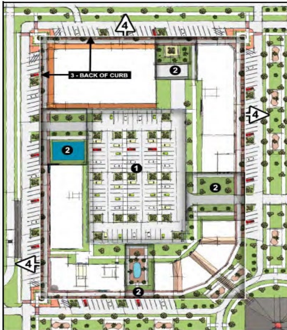
Sample Block Showing: (1) parking interior to the block; (2) limited, pedestrian scaled common areas screening the surface parking; (3) back of curb; and (4) block perimeter measured at the back of curb.
