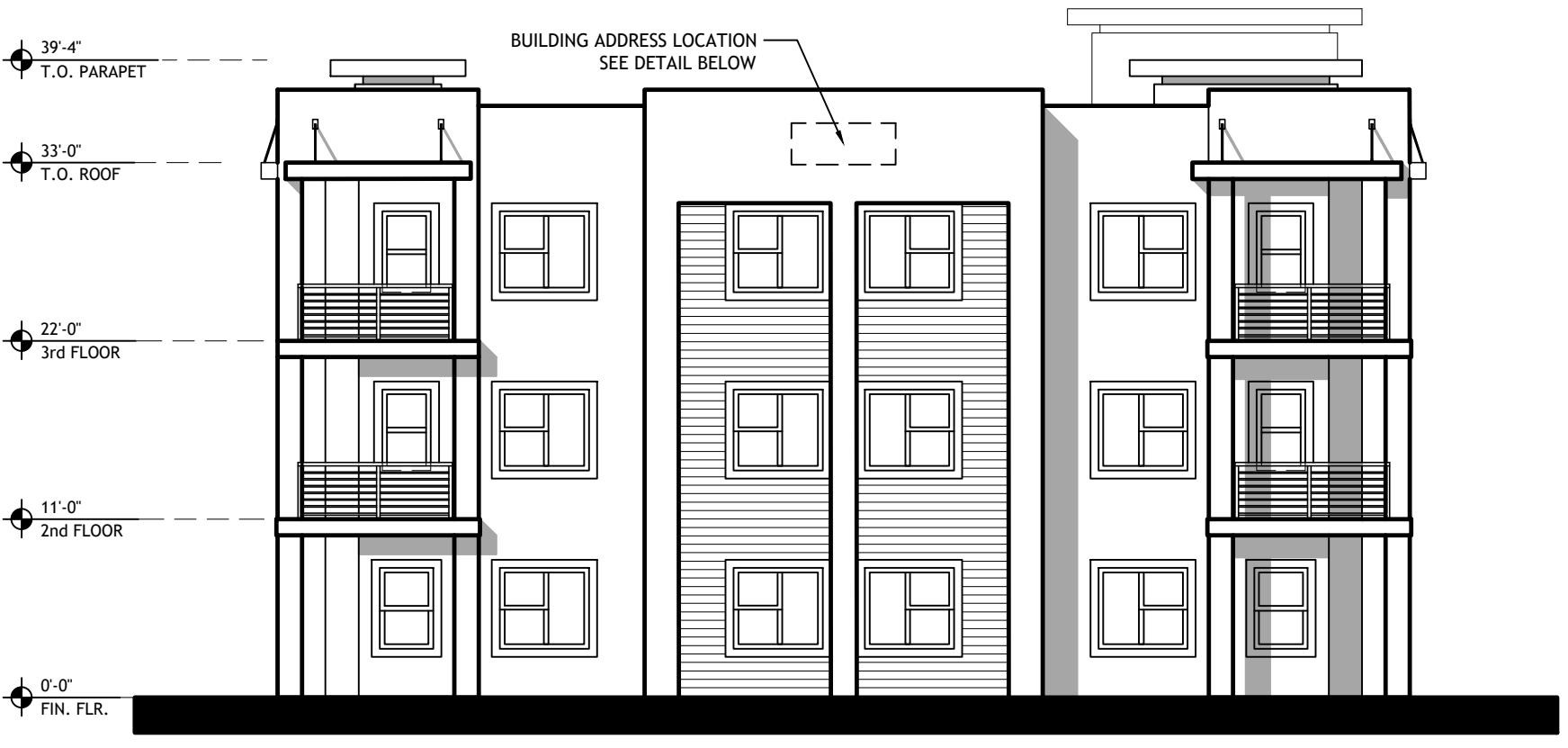
2 A25 SIDE ELEVATION BUILDING 'A'
