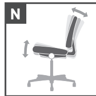
N. Multi-task control — Adjusts seat and back angles independently with a single lever (infinite locking within a fixed range).
