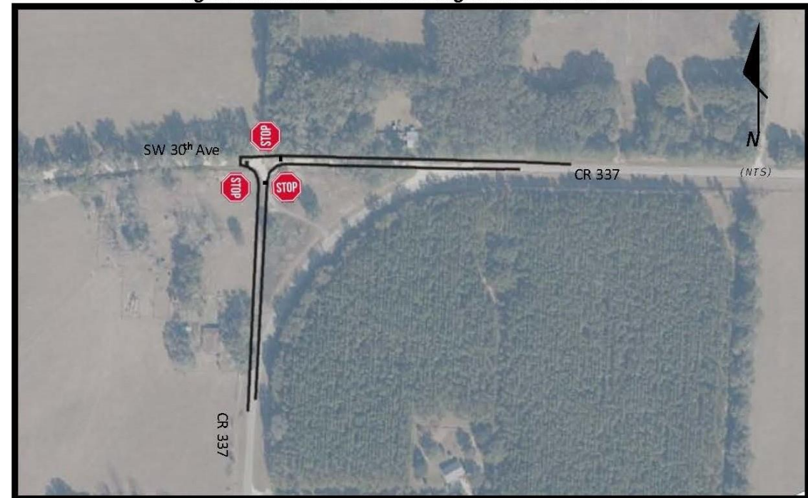
Figure 8: Scenario 2 - Curve Re-alignment at SW 30 th Ave
