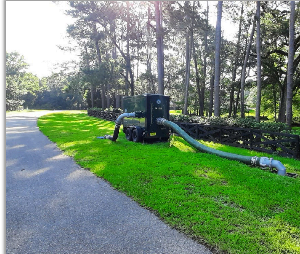
Single 8-inch pump with float switches
