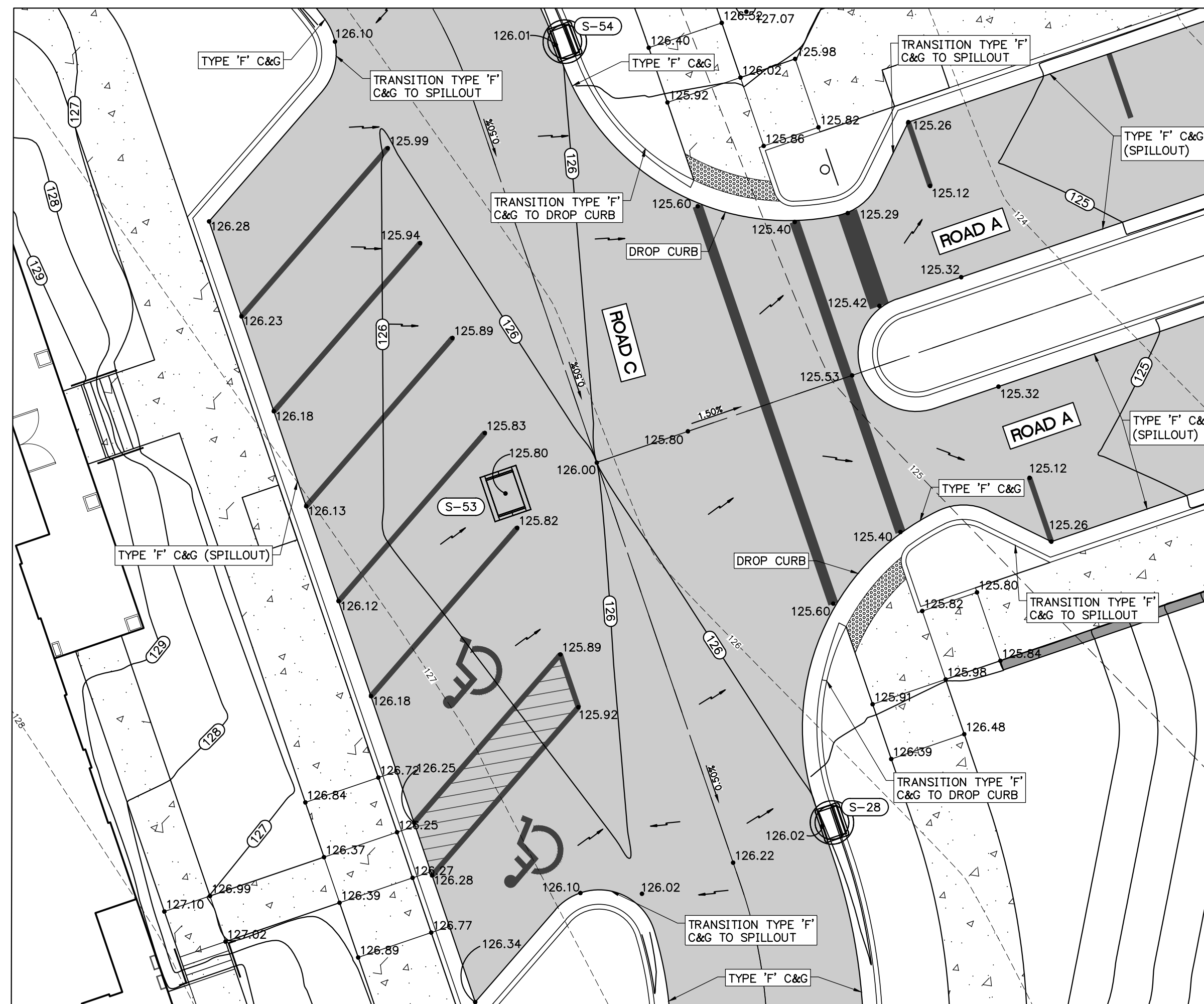
INTERSECTION - ROAD A AND ROAD C 1" = 10'
